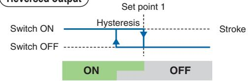
**2 Auto Switch Mode** Set point 1 is at the centre of the operating range (the range is approx. 3 mm).
