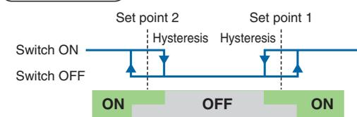
**4 2-Point Mode** Setting is only available in 2-point mode (IO-Link mode). Setting of set point 1 and 2 can change the ON and OFF position.
