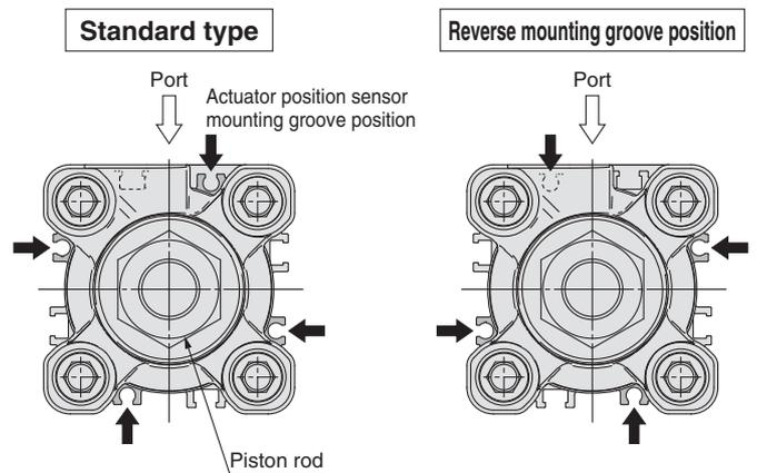
The mounting groove is reversed so that the actuator position sensor lead wire is not in the same direction as the piston rod.
