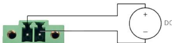
Figure 13: Connection of power supply
